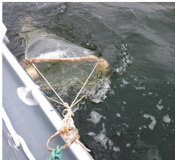
Fig. 3. Neuston net sampling. Net directly towed by boat
