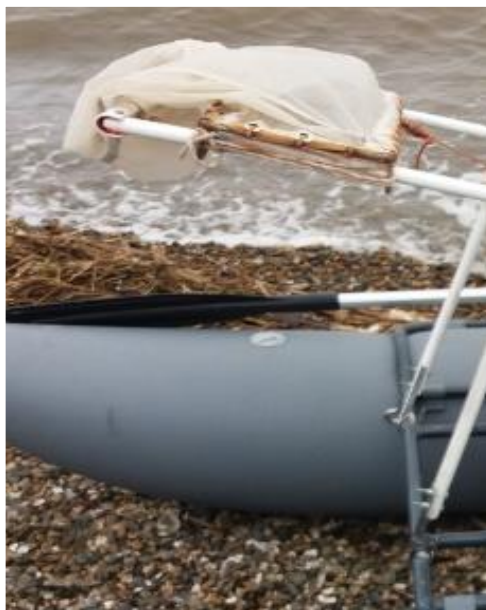
Fig. 4. Neuston net sampling. Net with adjustable frame is attached to a catamaran
